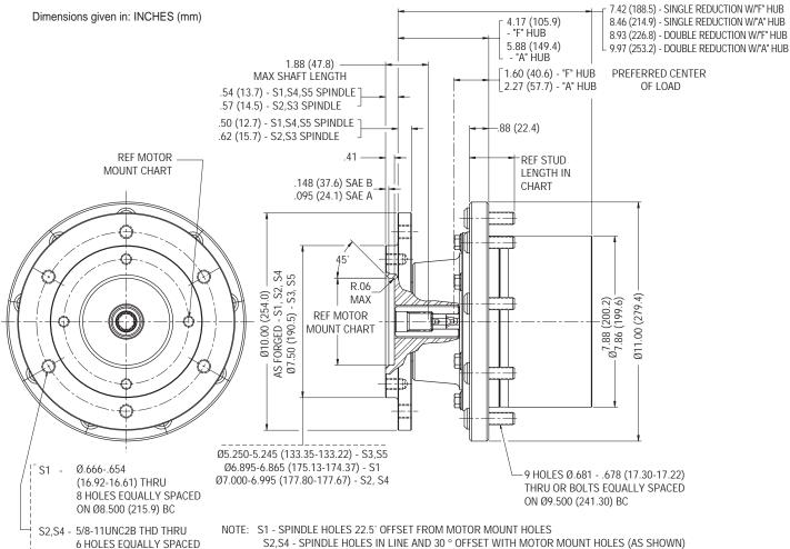
S3.S5 - 5/8-11UNC2B THD THRU 8 HOLES EQUALLY SPACED ON Ø6.500 (165.10) BC
