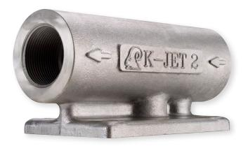
Sunfab Injector K-JET 2 is a basic technical solution for the recirculation of oil in closed hydraulic systems that is cost efficient and saves weight. Three models K-JET 2, cover the flows 160, 250 and 350 I/min.
