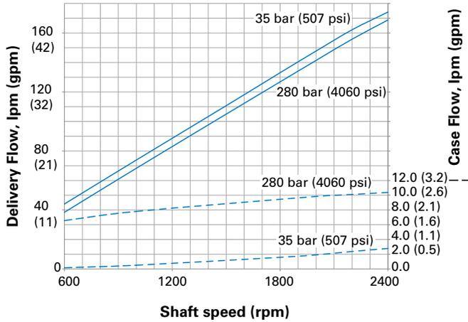
Input torque and case flow vs. speed @ stand-by and 49°C (120°F)
