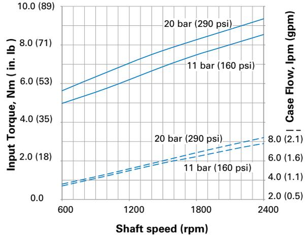
Input torque and case flow vs. speed @ Cut-off and 49°C (120°F)
