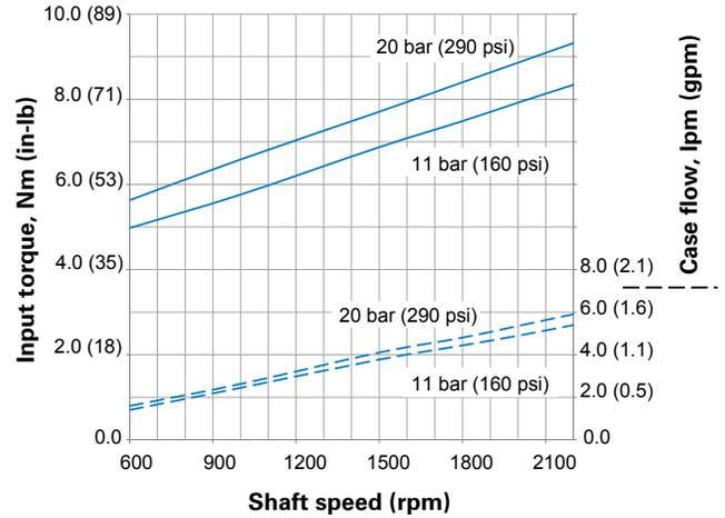
Input torque and case flow cut-off @ 49°C (120°F)
