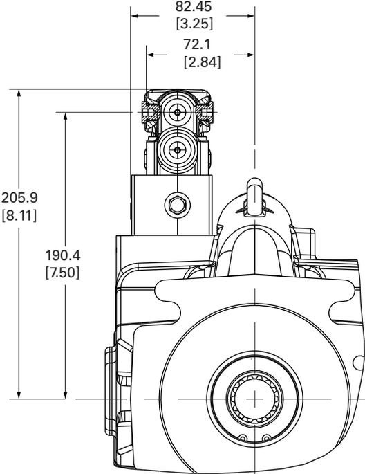
**Electronic Displacement Control (EDC)**
