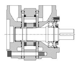
**BEARING LOADING** - The bearings in the 37 Series can accept radial load per the radial capacity charts to the right. Thrust loading is not recommended for the standard motor. For thrust-type applications, see the thrust capable motor bearing chart on the opposite page.
